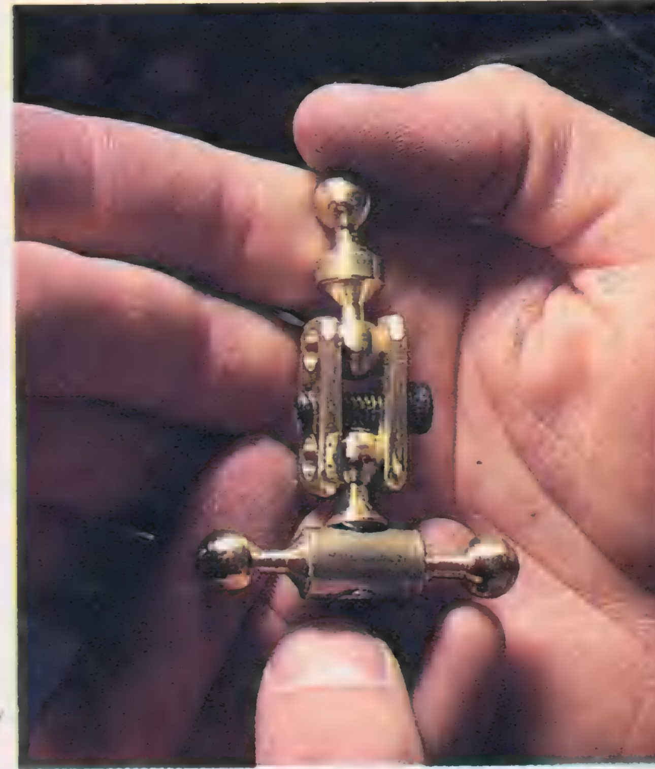
The finished joint is carefully broken in.
